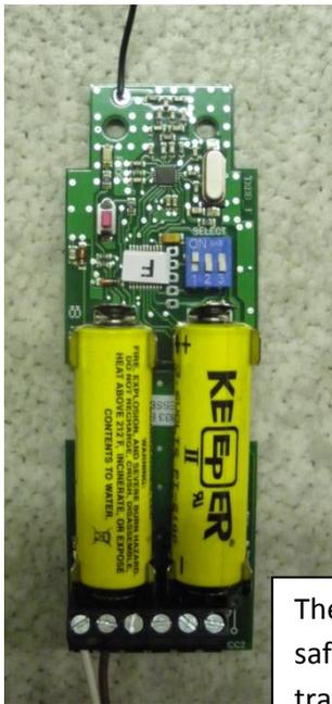
The photo shows the wire of the safety strip connected to the AERF transmitter
