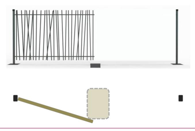
4. Take a new panel and a new post. Put fixators at both sides of the post and put the post in the hole.
