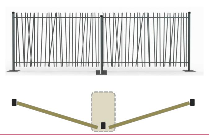
5. Now, simultaneously push the post and both panels back in place. Make sure the panels are taken by the fixators.
