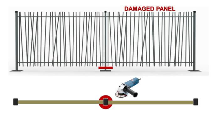
2. Remove the post by pulling/pushing the cut post and both panels simultaneously in one direction.
