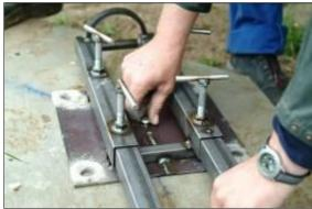
Position the gauge by means of putting a bolt or pen in the centre hole
