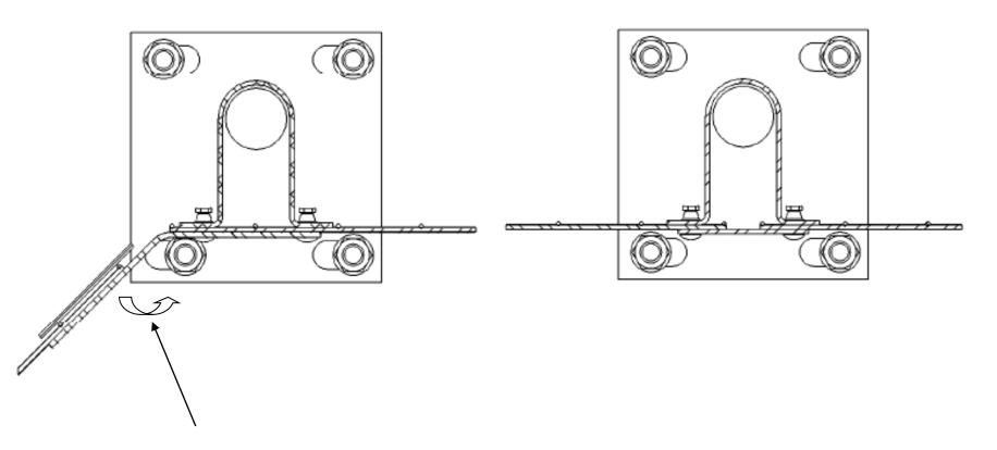
Sometimes it is necessary to position the anchor bolt at the other side of the slot in the base plate.
