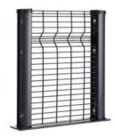
Bekafix® Secure posts are specifically designed and engineered to be used in combination with Betafence's panels. With Bekafix Secure, the fence is safely tucked behind the lip of the post, resisting against attempts to pry the panel looset. The panels are secured to the post with specialised fixators, firmly bolted through the post using stainless steel security bolts and shear-off nuts that protect against tampering.
