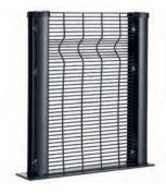
Bekafix® Secure posts are specifically designed and engineered to be used in combination with Betafence's panels. With Bekafix Secure, the fence is safely tucked behind the lip of the post, resisting against attempts to pry the panel loose from the post. The panels are secured to the post with our Mini Flat Max fixators, firmly bolted through the post using M6 stainless steel security bolts and shear-off nuts that protect against tampering.
